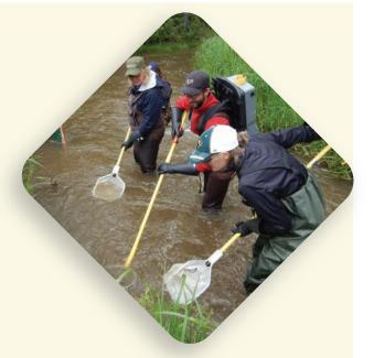
During the Electrofishing Certification Field Session, students will participate in a realistic field practicum, wearing and operating the backpack electrofishing unit, setting the machine for effective capture and completing sweeps and collection of fish. Students not operating the machine will participate in the field crew as dip netters and sampling crew.
